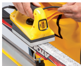
Top Finish Powder gebügelt Ironing Top Finish Powder Application à chaud de la poudre Top Finish Top Finish Powder messo a caldo con il ferro
