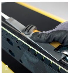
File edges with tools such as Edge Tuner or Side Angle WC Limare i bordi con strumenti quali Edge Tuner o Side Angle WC
