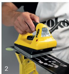
Iron in the wax evenly at the required temperature
