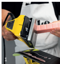
Applying the wax with the iron
