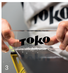
Allow to cool for at least 1 hour at room temperature and remove
