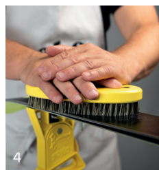
Brush off excess wax with a copper brush and polishing brush
