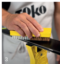
Allow to dry for approx. 25 minutes and polish with Base Brush Combi Nylon/Copper Lasciare asciugare per circa 25 minuti e lucidare con Base Brush Combi Nylon/Copper
