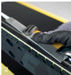
Kanten mit Tools wie Edge Tuner oder Side Angle WC feilen File edges with tools such as an edge tuner or side angle file guide
