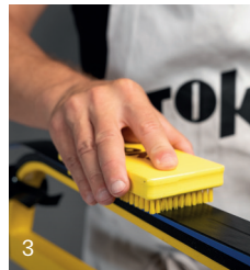
Mit Polishing Brush Liquid Paraffin polieren Polish liquid paraffin using a polishing brush
